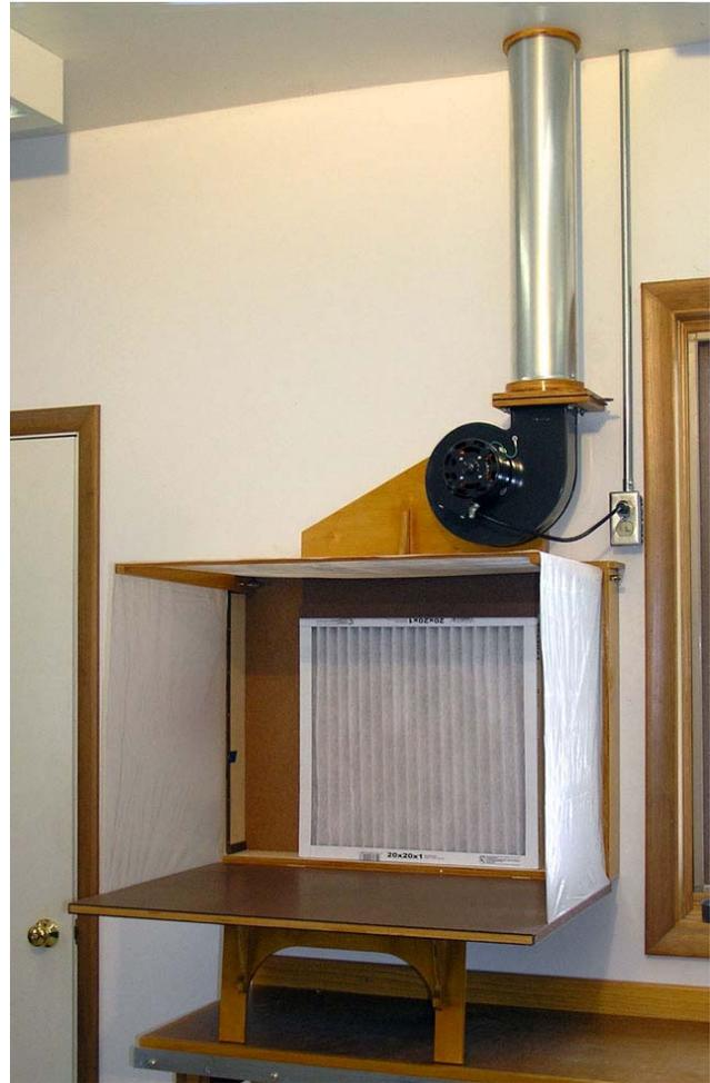
The throttle valve amounts to a tempered hardboard slider captured between two pieces of birch plywood.<sup>1</sup> The input opening is rectangular to match the blower; the output
