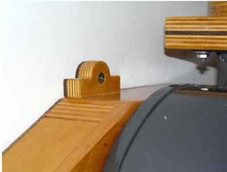
A scrap wood strip along the bottom of the cabinet baffles the crack that opens along the hinge line when the platform is lowered. This should protect my shop wall from escaping paint:
