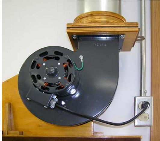
At this point, the booth was completely functional. Only a few little “naggers” remained to be cleaned up. I added a top mounting tab to stabilize the venturi against the shop wall; it’s very secure now:
