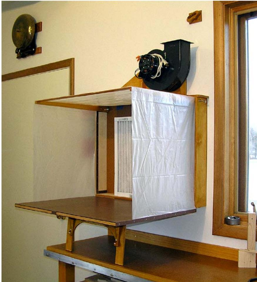
The walls and roof are a single piece of translucent vinyl plastic sheet, 3 mils thick. I cut a piece from a painter's drop cloth. The milky color of the vinyl allows plenty of light to enter, but diffuses it, so there are no harsh shadows in the painting area. This was an unplanned, but welcome bonus.
