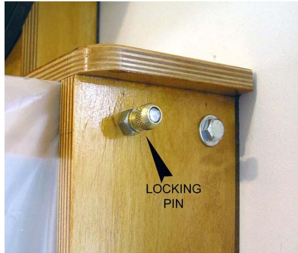
I hack sawed the heads off two more hex bolts to make the locking pins. The knurled brass "knobs" are just decorative nuts I found in my scrap box:
