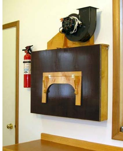
Looking ahead, the next task is to fabricate a throttle valve for the blower exhaust, so I can reduce airflow after spraying, while the paint is drying. I'm not anxious to expel expensively heated shop air into the cold outdoors unnecessarily.
