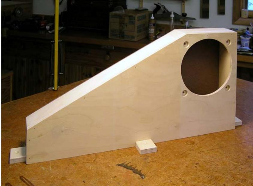
I used screws, rather than glue, to attach the back panel because it has to be removed for access to the blower mounting studs. The venturi operates at sub-atmospheric pressure, so I’m not too worried about any small leaks.
