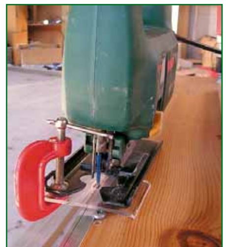
▲ A piece of perspex clamped to the bottom of the jig saw, with a hole just big enough for the saw blade, overcame the problem of holding down narrow (12mm) aluminium bar and cutting 2 mm off it.
